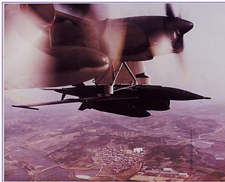
This is an AN/AQM-34Q reconnaissance drone designed and built by Teledyne Ryan Aeronautical. The “Q” and “R” models were made for long endurance, high altitude signals intelligence missions flown by the 350 th SRS from South Korea. All drone sorties began from an airborne launch off the wing of a highly modified Lockheed DC-130. This snapshot was taken over South Korea from the aircraft commander’s side window showing “Q” model #15 prior to launch. The special “Q” and “R” sorties will be covered in-depth in Chapter 13. Q-15 is now hanging from the ceiling of the U.S. Air Force Museum at Wright-Patterson AFB, Dayton, Ohio. (photo courtesy of Dave Matthews, circa 1972)
